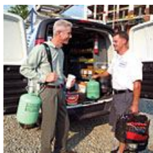
A simple, but safe, strap called the JugLugger allows easy toting of a refrigerant canister while still freeing up both hands for climbing ladders, carrying tools, or holding onto that all important first cup of coffee of the day.
